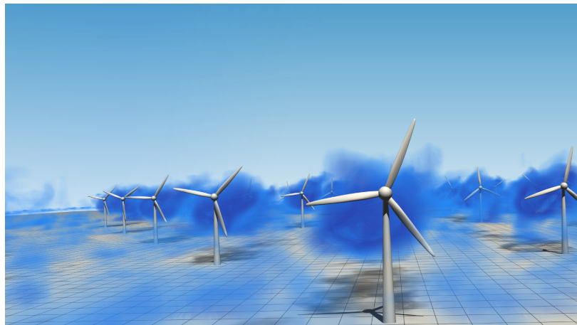
Figure 1: Visualization of Large Eddy Simulations of a wind farm by Srinidhi N. Gadde [9]
